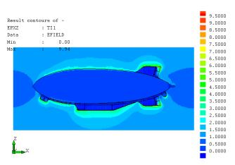
Figure 8. Typical Example of Airship Field Enhancement Factors for a Vertical Uniform Incident Static Electric Field for Triggered Lightning Evaluation
