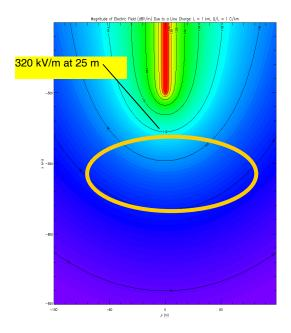
Figure 9. Fields from an Approaching Stepped Leader 1 km long and having 1 C/km linear charge density
