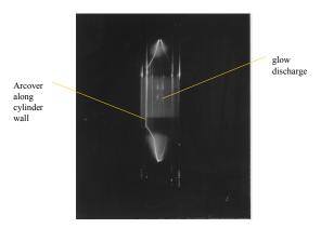
Figure 4. Helium Breakdown in Cylinder
