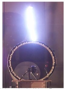
Figure 6. Lightning Leader Voltage Test on the 1:65 scale cylinder
